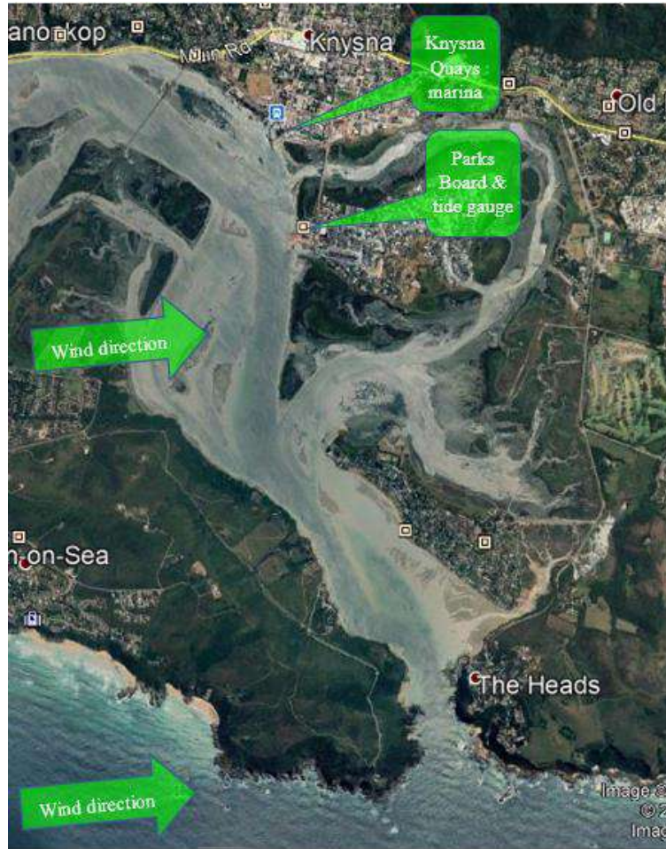
Figure Aa2-2: Westerly wind during the extreme water level event on 28 October 2019 at 16:00
