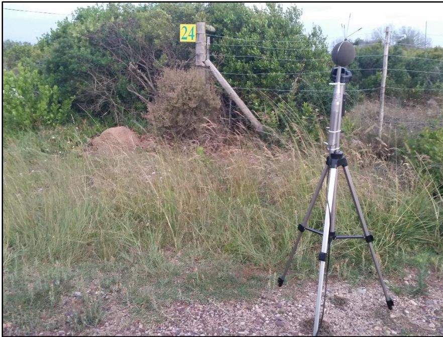
Figure 8: Sound level meter field installation
